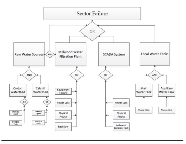
Figure 1. Fault Tree for the Village of Pleasantville Water Supply System.
