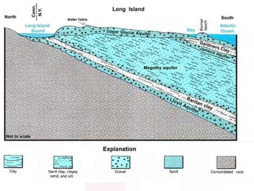
**Figure 1.** Geologic cross-section of the Long Island Aquifer System beneath Nassau County.<sup>13</sup>
