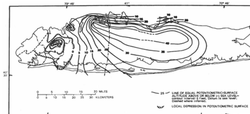
**Figure 4.** Depression in Potentiometric Surface in the Lloyd Aquifer, 1975.<sup>53</sup>
